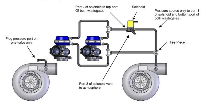
**Two port, twin solenoid, twin turbo connection Method (1)** (For controlling boost on a twin turbo, twin wastegate, twin solenoid turbo system, on a V configuration engine with high back pressure)
