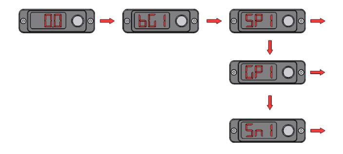
The E-Boost Street has the ability to control two levels of boost (BG1/BG2). The parameters that can be adjusted in each boost group are set point (SP1/SP2), gate pressure (GP1/GP2) and sensitivity (SN1/SN2). Set up the boost groups in the following order:
