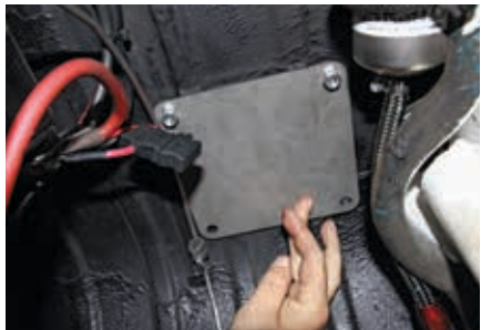
Flat roll bar plates are used to secure the rear bars to the parcel tray when the traction bars are not used. Use either to locate the rear bars by installing two screws and lightly tightening the nuts.
