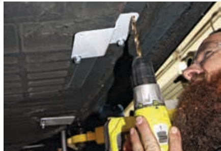
After all the pads have two bolts lightly securing them in place, it's time to drill the remaining holes and install all the bolts and nuts. You may have to massage the floorpan to get it flat enough.
