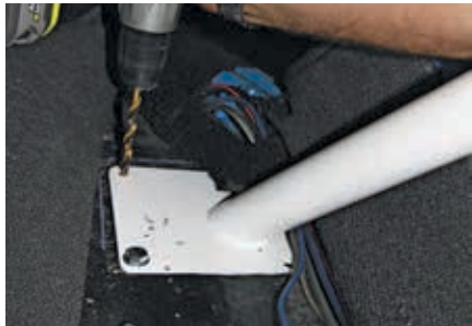
With the center and rear bars lightly secured, the door bars are next. Drill one hole and install the bolts with the nut lightly tightened, then install a second.
