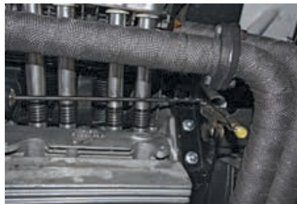
Here, Corey clamped the bar to the trans mount, and then used a long drill under the pushrod tubes to drill through the mount and mark where the traction bar should be drilled.
