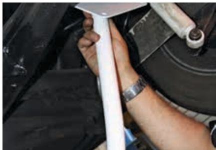
Because this Bug will receive the optional traction bars, the flat plates were removed and the bars added in their place. With all the components under the parcel tray it's a close fit.
