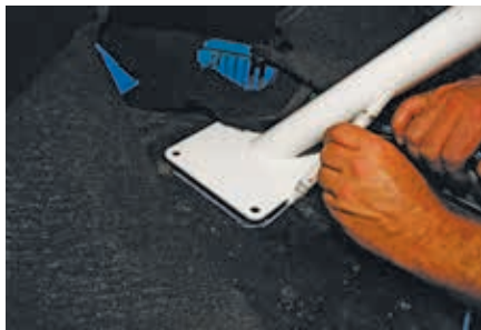
The factory tar boards needed to be removed, so the location of the mounting pad was marked. Once trimmed with a box knife, the tar board was removed from the mount location.
