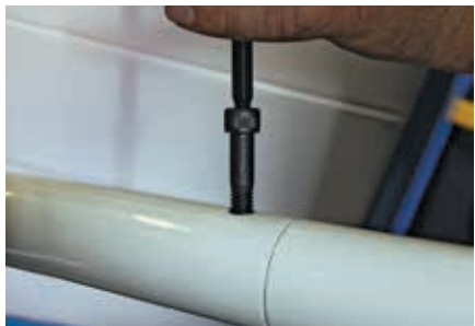
As with the rear bars, Philips head bolts are installed in the door bars, with the nuts left loose until later.
