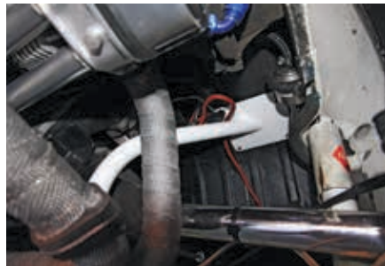
One of the last jobs is to bolt the traction bar to the trans mount, which can be quite difficult with the engine in place.
