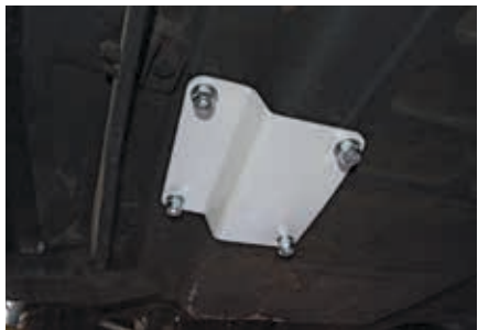
An installed roll bar plate. Note how this plate is bent to perfectly fit the shape of the floorpan.
