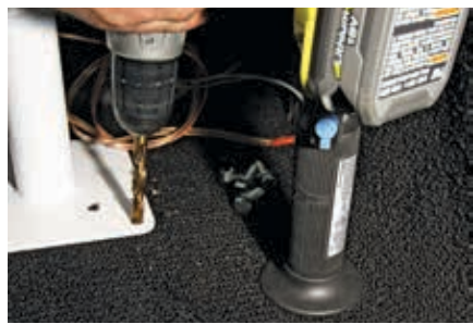
They decided to install the rear bar on top of the carpet, but you know how a drill bit can grab a strand of material, leaving a line of missing carpet! Check out the sidebar on heating your drill bit!
