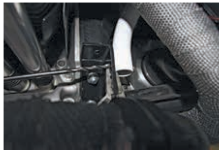
A close-up of the drill shows how it's at an angle, so just use the long drill to mark the location on the traction bar.
