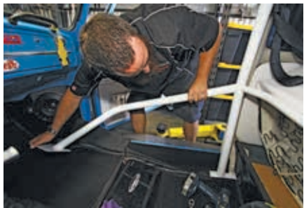
Here, Powerhaus' Corey Siler puts the passenger side door bar in place. For this installation they will be placing the roll bar mounting pads under the carpet.
