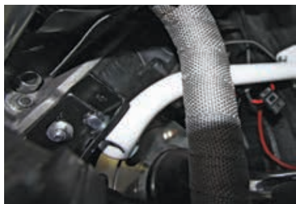
Use the 3/8-inch drill bit to finish the hole in the transaxle mount, then install the bolt and tighten the nut.
