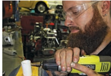
Now remove the traction bar from the car, secure in a vise, and drill the 3/8-inch hole at the mark as square as possible.
