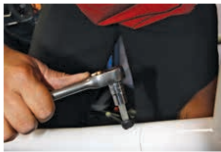
The last thing to do is go back and fully tighten all the roll bar bolts, both at the slip joints and all the plates.
