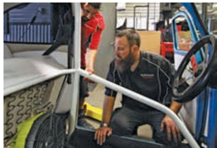
Corey and Moises Guerrero checking the alignment of the holes in the door bar. Correct alignment will ensure that the pads sit flat on the floorpan.
